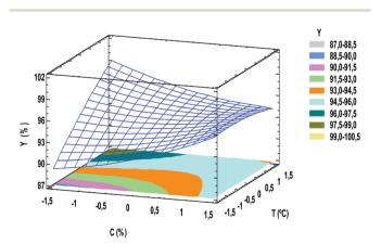
Fig. 3 Response surface and contour plot of ethyl ester yield as a function of catalyst concentration and temperature.
