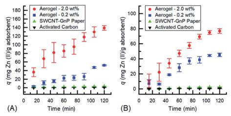
Fig. 4 Time dependent adsorption for removal of adsorbate (Zn(u)) with initial concentrations of (A) 0.5 mg mL<sup>-1</sup> and (B) 0.1 mg mL<sup>-1</sup> by carbon nanomaterial (CNM)-based aerogels of (●) 2.0 wt% and (■) 0.2 wt%, (▲) SWCNT-GnP paper, and (▼) activated carbon
