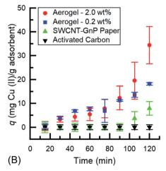
Fig. 3 Time dependent adsorption for removal of adsorbate (Cu(III)) with initial concentrations of (A)  $0.5 \text{ mg mL}^{-1}$  and (B)  $0.1 \text{ mg mL}^{-1}$  by carbon nanomaterial (CNM)-based aerogels of ( $\bullet$ ) 2.0 wt% and ( $\blacksquare$ ) 0.2 wt%, ( $\triangle$ ) SWCNT-GnP hybrid paper, and ( $\blacktriangledown$ ) activated carbon.
