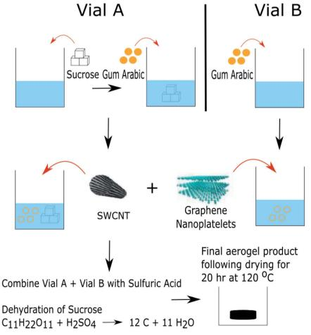
Scheme 1 Preparation process for carbon nanomaterial-based aerogels
