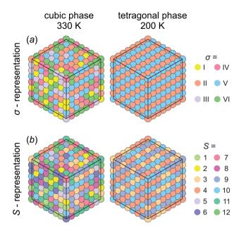
Fig. 5 Snapshots of simulations of our model performed at 330 K (cubic phase) and 200 K (tetragonal phase). The cation states are represented in the (a)  $\sigma$ - and (b) S-representations. The long-range order is clearly observed in the tetragonal phase ( $\sigma$  = II (S = 3,4) and  $\sigma$  = V (S = 9,10) states). Simulation parameters:  $\varepsilon_1$  = 21 meV,  $\varepsilon_2$  = 12.6 meV, L = 20.
