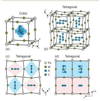
Fig. 1 Structure of FAPbBr<sub>3</sub> in the (a) cubic and (b-d) tetragonal phases. There are 48 and 4 equivalent orientations (indicated by transparent atoms) of FA cation in the cubic and tetragonal phase, respectively. Color coding in (d) corresponds to the colors of the rhombic channels in (c). Structural data taken from ref. 27.
