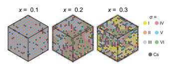
Fig. 7 Snapshots of simulations of our model for different Cs<sup>+</sup> ion concentrations. The FA cation states are represented in the  $\sigma$ -representations. Simulations are performed by starting from the disordered phase and gradually lowering the temperature significantly below  $T_0$ . A multidomain structure is observed at the higher mixing levels. Simulation parameters:  $\varepsilon_1$  = 21 meV,  $\varepsilon_2$  = 12.6 meV,  $\varepsilon_{Cs}$  = 31.5 meV, L = 16.
