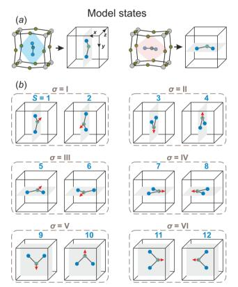
Fig. 2 (a) Examples of mapping of the experimental FA cation orientations to the corresponding model states. (b) Twelve states (S =  $1, \dots, 12$ ) of FA cation considered in our model. The electric dipole moment ( $C_2$  symmetry axis) of each state is denoted by the red arrow. The cations situated within the same plane and having an opposite dipole moment are assigned to the same  $\sigma$ -state enumerated by the Roman numerals ( $\sigma = I, \dots, VI$ ).
