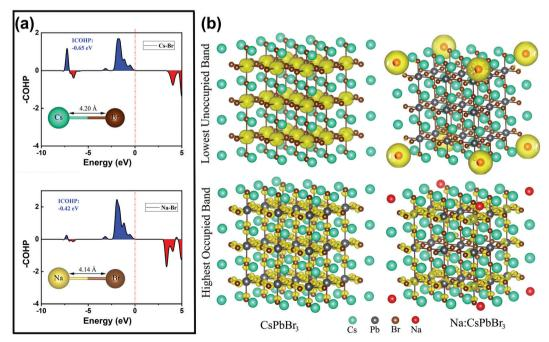
Fig. 5 (a) COHP plots of Cs-Br and Na-Br interactions for CsPbBr<sub>3</sub> (top) and Na<sup>+</sup>-doped CsPbBr<sub>3</sub> (bottom). (b) The corresponding isosurfaces of the charge density of the highest occupied band (bottom) and lowest unoccupied band (top) in CsPbBr<sub>3</sub> and Na<sup>+</sup>-ion-doped CsPbBr<sub>3</sub>.
