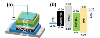
Fig. 6 (a) A schematic illustration and (b) flat-band energy level diagram of the CsPbBrz QLED device.
