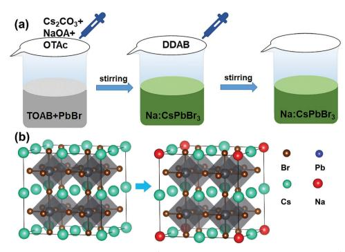
Fig. 1 (a) A schematic illustration of the synthesis procedure of Na<sup>+</sup>-doped CsPbBr<sub>3</sub> QDs. (b) A representative model of Na<sup>+</sup>-doped CsPbBr<sub>3</sub> QDs showing the replacement of some Cs positions with Na atoms
