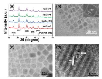
Fig. 2 (a) XRD patterns of the as-synthesized Na<sup>+</sup>-doped CsPbBr<sub>3</sub> QDs with different Na/Cs ratios. TEM images of (b) CsPbBr<sub>3</sub> and (c) representative Na+-doped CsPbBr<sub>3</sub> QDs (Na/Cs = 1:3). (d) A HRTEM image of a typical Na<sup>+</sup>-doped CsPbBr<sub>3</sub> QD. The inset of (b) shows a HRTEM image of one CsPbBr3 QD
