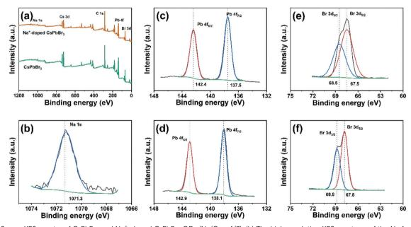
Fig. 3 (a) Survey XPS spectra of CsPbBr<sub>3</sub> and Na<sup>+</sup>-doped CsPbBr<sub>3</sub> QDs (Na/Cs = 1/3). (b) The high-resolution XPS spectrum of the Na 1s signal in the Na<sup>+</sup>-doped CsPbBr<sub>3</sub> QDs. (c-f) High-resolution XPS spectra corresponding to the Pb and Br elements in doped and undoped CsPbBr<sub>3</sub> QDs. The black curves represent the original data, the blue and red curves are the fitting peaks, and the green lines are the background.
