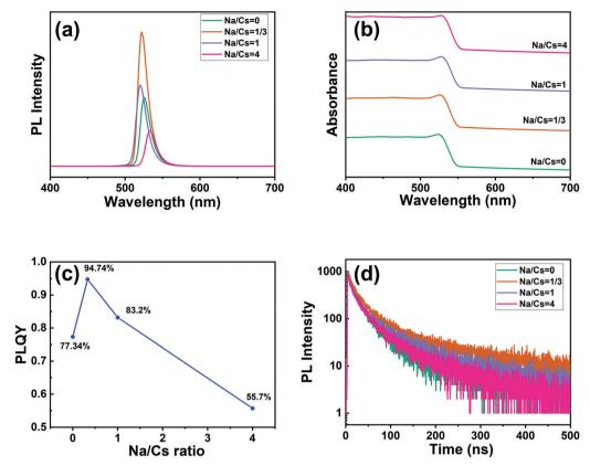
Fig. 4 (a) PL spectra (excited by 365 nm light), (b) absorption spectra, (c) PLQY data, and (d) time-resolved PL decay curves of CsPbBr<sub>3</sub> and Na<sup>+</sup>-doped CsPbBr3 QDs.
