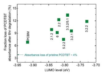
Fig. 2 Fraction of initial polymer absorbance at 571 nm that is lost after 6 h exposure to AM 1.5G illumination in air for each PCDTBT:fullerene blend films as a function of the measured LUMO level of the acceptor. Also indicated is the absorbance loss of the pure polymer film. The absorbance measurements of neat fullerene films are not shown since there was no significant change after 6 h illumination, in agreement with results in the literature.30
