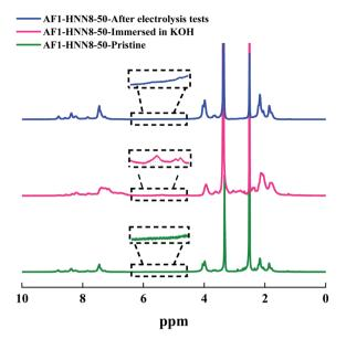
Fig. 6 <sup>1</sup>H NMR spectra of AEM HNN8-50, in the pristine form (lower), after storage in 2 M KOH at 90 °C for one month (mid), and after the electrolysis test (upper). The data were recorded in DMSO- $d_6$ .
