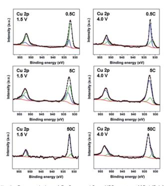
Fig. 3 Deconvolution of Cu  $2p_{3/2}$  and  $2p_{1/2}$  XPS spectra of  $[CuL(Py)_2]_n$  electrodes at various rates. 0.5C (top), 5C (middle) and 50C (bottom) at end of discharge (1.5 V, left) and end of charge (4.0 V, right) (green: Cu(0); blue: Cu(I)).
