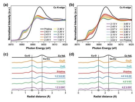
Fig. 4 XAS of  $[CuL(Py)_2]_n$  electrodes: (a) and (b) in situ Cu K-edge XANES patterns during discharge and charge at 20 mA  $g^{-1}$  ( $\sim 0.08C$ ), respectively. (c) and (d) Ex situ Cu K-edge EXAFS patterns at three different rates (0.5C, 5C and 50C) at end of discharge (1.5 V) and end of charge (4.0 V), respectively (with Cu foil, Cu<sub>2</sub>O and CuO as references).
