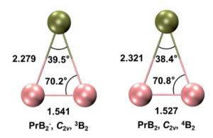
Fig. 2 The global minimum structures of PrB<sub>2</sub><sup>-</sup> and PrB<sub>2</sub> calculated at the PBEO/TZP level using ADF program. The bond lengths are given in Å and the bond angles are given in degree (°). Colour codes for atoms: olive-Pr; pink - B
