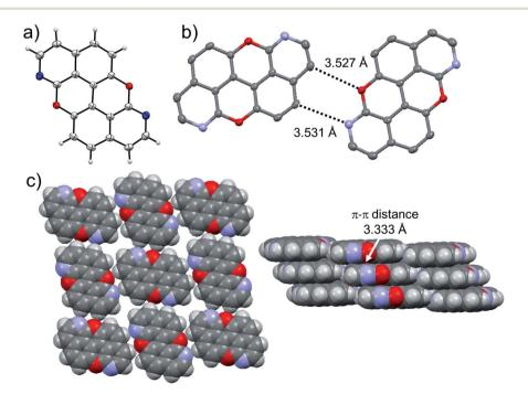
Fig. 8 Single-crystal X-ray structure of 1,7-N,N-PXX. ORTEP representation (a) and structure of two isolated molecules engaging into H-bonds (b) depicting a multilayer-type organisation of  $\pi$ - $\pi$  stacked supramolecular H-bonded sheets (c). Space groups:  $P2_1/c$ . Atom colours: red O, blue N, grey C, white H.
