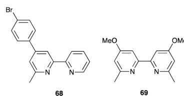
Scheme 24 Structures of ancillary ligand 68 , and of ligand 69 used in a Cu 2+ /Cu + redox shuttle.
