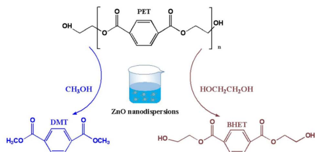
Fig. 11 Nano-ZnO dispersion catalyzed depolymerization of PET.
