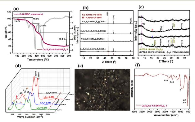
Fig. 4 (a) TGA spectrum of MOF precursor-4 conversion to catalyst  $Co_9S_8/Co-N_x/CoNi/Ni_3S_2@CNS-4$ , (b and c) XRD patterns of electrocatalysts  $CoS/Co-N_x/CoNi/NiS@CNS$ , (d) Raman spectra of catalysts 1–4, (e) Raman image (laser at 532 nm) of a filter showing the distribution of graphitic carbon, and (f) the FT-IR spectrum of  $Co_9S_8/Co-N_x/CoNi/Ni_3S_2@CNS-4$ .
