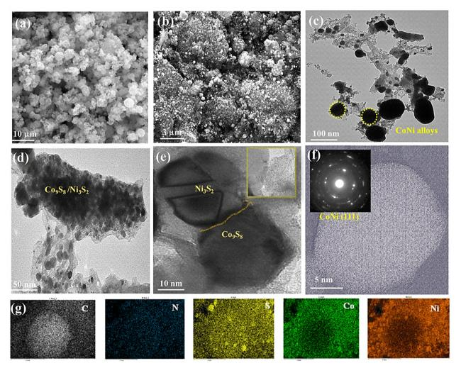
Fig. 3 (a) FE-SEM images of MOF precursor-4 and that (b) after calcination of the corresponding dandelion flowers like Co<sub>9</sub>S<sub>8</sub>/Co-N<sub>x</sub>/CoNi/  $Ni_3S_2$ @CNS-4 catalyst, (c-e) TEM images of  $Co_9S_8/Co-N_x/CoNi/Ni_3S_2$ @CNS-4,  $Co_9S_8/Ni_3S_2$  and their heterojunction, (f) TEM image of CoNi alloy nanoparticle; inset show derived fast Fourier transform SAED patterns, and (g) EDS mappings for carbon (C), nitrogen (N), sulphur (S), cobalt (Co) and nickel (Ni).
