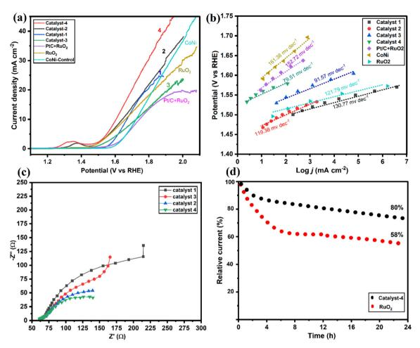
Fig. 7 Electrocatalytic OER performances: (a) LSV curves of  $CoS/Co-N_x/CoNi/NiS@CNS$  1–4, commercial  $RuO_2$  and  $Pt/C + RuO_2$  in  $N_2$ -saturated 0.1 M KOH, (b) Tafel plots of LSV curves of catalysts 1–4,  $RuO_2$  and  $Pt/C + RuO_2$ , (c) EIS spectra of catalysts 1–4, and (d) chronoamperometric responses of  $Co_0S_8/Co-N/CoNi/Ni_xS_2@CNS-4$ , and commercial  $RuO_2$  in  $N_2$ -saturated 0.1 M KOH solution.
