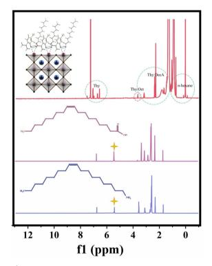
Fig. 7 <sup>1</sup>H NMR spectra of NADES-CsPbBr<sub>3</sub> PNCs, OA and OAm.
