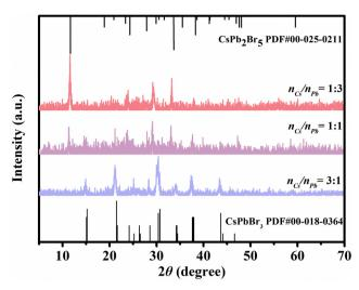
Fig. 5  $\,$  XRD patterns of PNCs synthesized with different molar ratios of CsBr and PbBr $_2$ .
