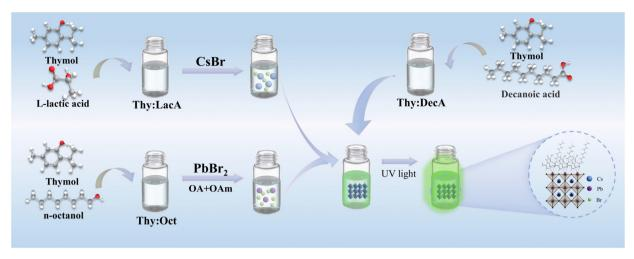
Fig. 1 Schematic illustration of synthetic procedure for NADES-CsPbBr<sub>3</sub> PNCs.
