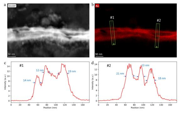
Fig. 12 STEM-EDX analysis of a sample taken in an adjacent region to the Bishop sample: (a) high-angle annular dark-field (HAADF) image and (b) EDX Au map of a Zwischgold leaf cross-section; (c and d) EDX line profile across the leaf along the green arrows in (b).
