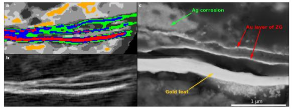
Fig. 9 (a) A segmented and (b) raw PXCT tomogram slice for *Nicolaus Border*; (c) SEM image of a microtomed cross-section of the "Nicolaus Border" sample labelled with observations from EDX analysis. Scale bar applies to all images.
