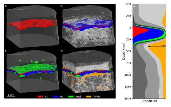
Fig. 5 PXCT 3D images of the Mary sample showing the addition of (a) Au, (b) Ag (with transparent voids), (c) "silver corrosion products", and (d) other segments (see Fig. 7 for segmentation details). (e) Stack plot of the depth profile of the sample, aligned to the main layer of the Au segment.
