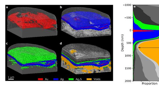
Fig. 4 PXCT 3D images of the 35-year old Zwischgold sample showing the addition of (a) Au, (b) Ag (with transparent voids), (c) "silver corrosion products", and (d) other segments (see Fig. 3 for segmentation details). (e) Stack plot of the depth profile of the single-layered section of the sample, aligned to the main layer of the Au segment.
