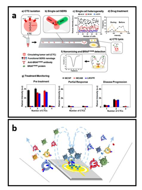
Fig. 11 Schematics of the small devices with SERS-based sensors: (a) SERS-based microfluidic immunoassay for in situ characterization of single CTCs, adapted from ref. 214 with permission from the American Chemical Society, copyright 2021; (b) nano-mixing-enhanced EVs subpopulation characterization platform adapted from ref. 215 with permission from the American Chemical Society, copyright 2021.
