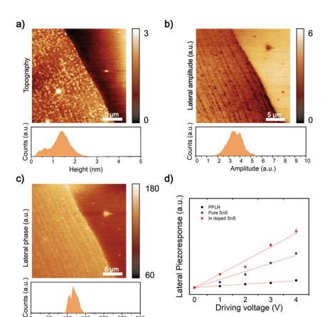
Fig. 5 2D SnS with 6.4 at% In doping lateral piezoelectric response. (a) The AFM morphology and the 2D layer. (b) 6.4 at% In alloy concentration single layer Lateral amplitude, histogram with the attached picture. (c) 6.4 at% In doped in SnS lateral phase, the inset is a histogram. (d) The lateral piezoelectric response of 6.4 at% In doped in SnS single layer nano-film, pristine and PPLN to different driving voltages. Error bars indicate the standard deviation of the measurement.
