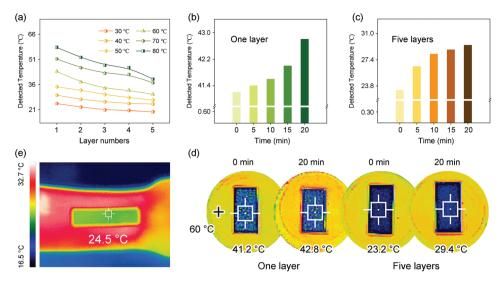
Fig. 7 (a) Variation of the temperature detected on the upper surface of the NF@Co/C architecture with the number of layers at different heating temperatures. Variation of the temperature detected of (b) one-layer and (c) five-layer samples with heating time, as well as (d) the corresponding thermal infrared images. (e) Thermal infrared image of the NF@Co/C architecture placed on the arm.
