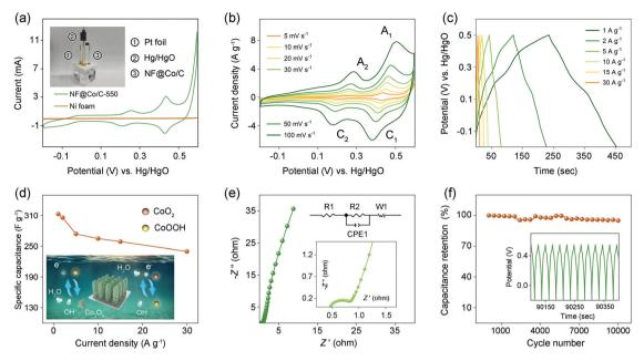
Fig. 8 (a) CV curves of Ni foam and NF@Co/C-550 sample at a scan rate of 5 mV s<sup>-1</sup>. Inset is a three-electrode system. (b) CV curves of NF@Co/ C-550 sample at different scan rates. (c) GCD curves at different current densities. (d) Specific capacitance. Inset is the schematic illustration for electrode reaction. (e) Nyquist plots and the corresponding equivalent circuit. (f) Cycling performance at a charge-discharge current density of  $10 \text{ A g}^{-1}$ .
