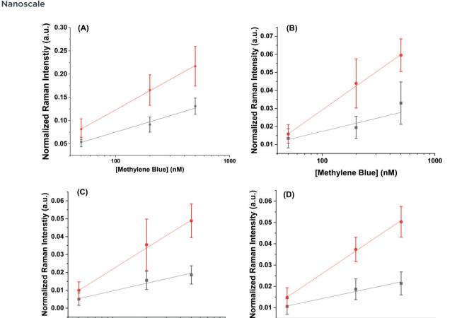
Fig. 5 The signal profile from 50-500 nM for the peaks at (A)  $447 \text{ cm}^{-1}$  (B)  $770 \text{ cm}^{-1}$  (C)  $1390 \text{ cm}^{-1}$  and (D)  $1620 \text{ cm}^{-1}$  for the AuNR@Full (black) and the AuNR@Ends (red). These points are fitted to a logarithmic equation and the slope was extracted to determine which concentration causes the SERS intensity to be higher than the intensity with no methylene blue added plus 3 standard deviations.
