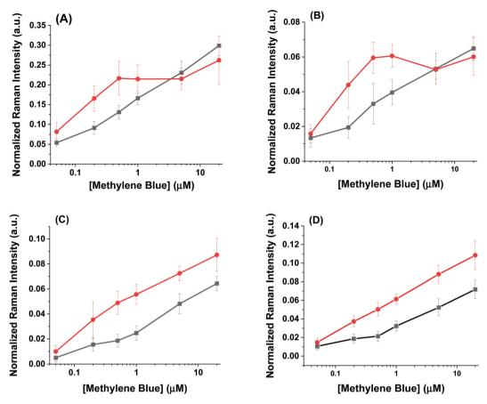
Fig. 4 Normalized intensity of different methylene blue Raman peaks relative to internal ethanol Raman peaks for (A) 447 cm<sup>-1</sup> (B) 770 cm<sup>-1</sup> (C) 1390 cm<sup>-1</sup> (D) 1620 cm<sup>-1</sup>. The AuNR@Full and the AuNR@End colloidal substrates are shown in black and red, respectively.
