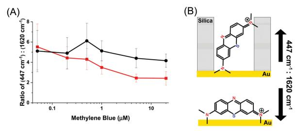
Fig. 6 (A) The ratio of the peaks at 447 cm<sup>-1</sup>:1620 cm<sup>-1</sup> for full silica (black) and end coated (red) AuNRs following exposure to varying amount of methylene blue. (B) A representation of the molecular orientation when the analyte is (top) in a pore and (bottom) not in a pore. The yellow represents the gold surface and the gray background represent the silica/pore channels.
