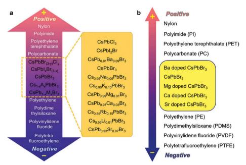
Fig. 7 Triboelectric series of CsPbBr<sub>3</sub> perovskite and its Cs-site and Pb-site substituted compounds. Qualitative triboelectric series of the (a) pristine CsPbBr<sub>3</sub>, Cs<sub>1-x</sub>A<sub>x</sub>PbBr<sub>3</sub> and (b) CsPb<sub>1-x</sub>M<sub>x</sub>Br<sub>3</sub> perovskites. Reproduced with permission from ref. 87 and 90. Copyright 2020 from Elsevier and Copyright 2020 from Royal Society of Chemistry.
