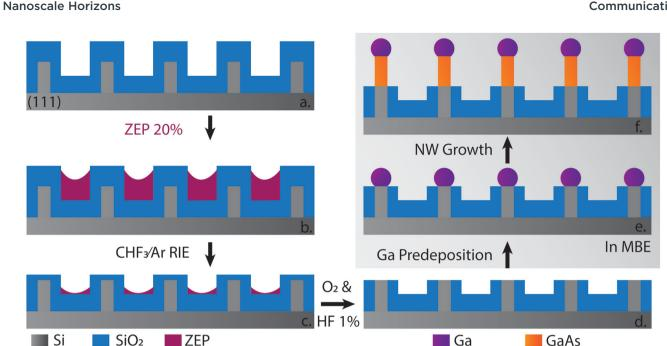
Fig. 1 Schematic detailing the fabrication steps of SiO<sub>2</sub>/Si(111) pillars for self-catalyzed VLS GaAs NW growth. (a and b) The resist spin-coating process, (b and c) The RIE step and (c and d) the last wet etching before MBE loading. (e) Shows the very critical Ga predeposition step followed by (f) showing NW growth.
