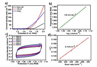
Fig. 3 (a) Polarization curves of PS-78 and the substrate (GS) at a scan rate of 5 mV s<sup>-1</sup>, (b) Tafel plot of PS-78, (c) cyclic-voltammetry curves of PS-78 at different scan rates (200–300 mV s<sup>-1</sup>) and (d) double layer charge capacitance ( $C_{dl}$ ) of PS-78.
