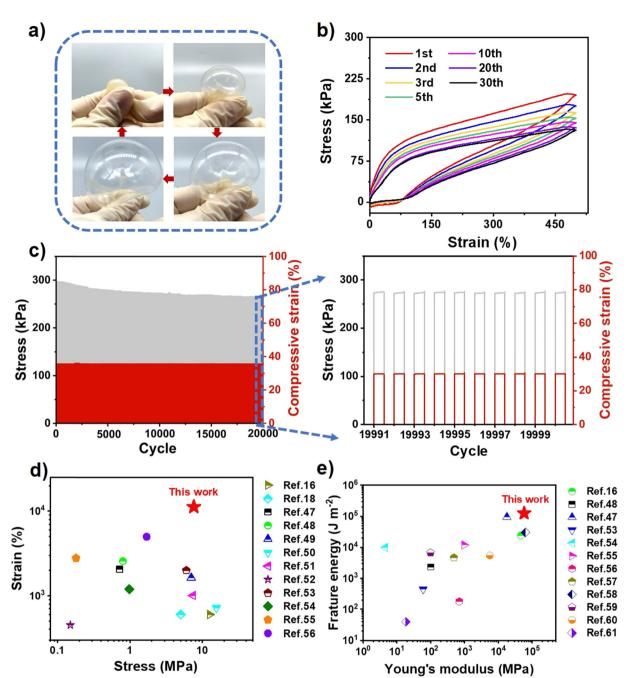
Fig. 4 Mechanical properties of UiO-66-ionogels. (a) UiO-66-ionogel (2 × 2 cm²) could be inflated by nitrogen and demonstrated excellent toughness. (b) UiO-66-ionogel could be compressed over 20 000 cycles at 30% strain (with 30 s intervals). (c) Cyclic stress-strain curves of the UiO-66-ionogel at 500% with 1 min intervals. (d and e) Comparison of the mechanical properties (strain, stress, Young's modulus, and fracture energy) between UiO-66ionogels and recently reported ionogels.
