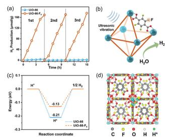
Fig. 4 (a) Three cycles of time-dependent H<sub>2</sub> evolution curves over UiO-66 and  $UiO-66-F_4$  under ultrasonic vibration. (b) Schematic illustration of the mechanism of piezocatalytic H<sub>2</sub> production from water over the UiO-66-F<sub>4</sub> via harvesting vibration energy. (c) Gibbs free energy ( $\Delta G_{H^*}$ ) diagram for hydrogen adsorption on UiO-66 and UiO-66-F<sub>4</sub>. (d) Most stable atomic configurations of hydrogen adsorption on UiO-66-F<sub>4</sub>.
