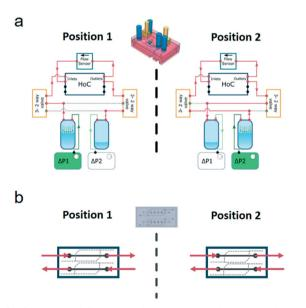
Fig. 2 Operation of flow control system for recirculation of culture medium with unidirectional flow in the connected heart-on-chip. a) Overview of the fluidic circuit flow path between the different MFBBs and the respective flow direction in two respective positions of the valves (left and right), b) Overview of flow direction inside the hearton-chip device demonstrates identical flow patterns in both positions of the system.
