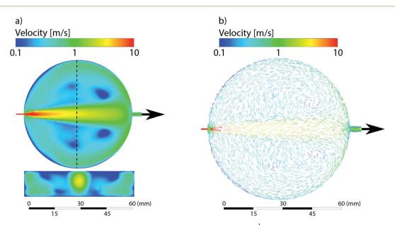
Fig. 5 Gas simulations for a cylindrical cell with a 0.4 mm inlet at a gas flow of 0.9 L min<sup>-1</sup> of He. (a) Gas profile from above at the height of the exit with the cross section below, indicated by the dashed line. (b) Vector plot showing the directions of gas flows.
