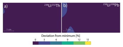
Fig. 7 Contour plots of normalized mean elemental ratios of (a)  $^{238}$ U/ $^{232}$ Th ratio and (b)  $^{238}$ U/ $^{208}$ Pb ratio for bulk analysis using the PFAC and 2.5 meter PVC tubing to smooth the aerosol. Plots were calculated using 32 different positions on the sample stage for low dispersion laser ablation, corresponding to the area of a standard microscope slide. View representing the entire sample stage from above.
