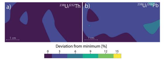
Fig. 4 Contour plots of median (a) <sup>238</sup>U/<sup>232</sup>Th ratio and (b) <sup>238</sup>U/<sup>208</sup>Pb ratio over 200 resolved laser pulses calculated using 32 different positions on the sample stage for low dispersion laser ablation, corresponding to the area of a standard microscope slide. Data were acquired using a total of 8 different NIST SRM 612 disks. View representing the entire sample stage from above.
