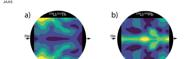
Fig. 3 Contour plots of (a)  $^{238}$ U/ $^{232}$ Th ratio and (b)  $^{238}$ U/ $^{208}$ Pb calculated using 28 different positions on a total of 6 different NIST SRM 612 disks. Only the upper halves were measured within the cylindrical ablation cell, while the lower halves were mirrored along the center line due to symmetrical gas flows. The instrument was optimized at the centermost position for a  $^{238}$ U/ $^{232}$ Th ratio of 1.00.
