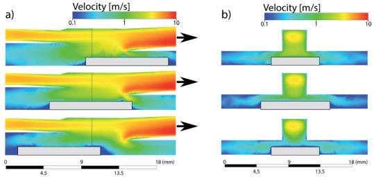
Fig. 6 Gas flow simulations for the PFAC for three different sample positions (grey) at a He flow rate of  $1.6 \, L \, min^{-1}$  and Ar flow rate of  $0.8 \, L \, min^{-1}$ . The sample (grey) is positioned  $0.8 \, mm$  below the opening. (a) Side view with the arrow representing the direction of the ICP. (b) Cross section at the dashed line from (a).
