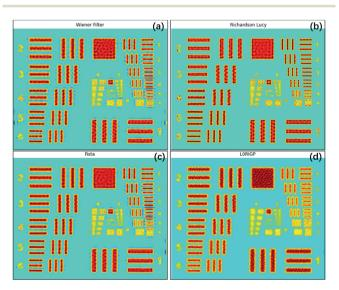
Fig. 5 Results of four image restoration methods: (a) Wiener filter, (b) Richardson-Lucy, (c) fast iterative shrinkage-thresholding algorithm (FISTA), and (d) blind deblurring with L0-regularized intensity and gradient prior (LORIGP).
