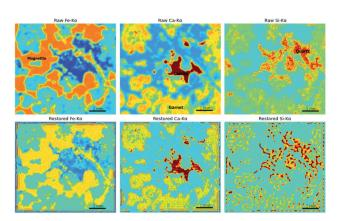
Fig. 9 XRF images of an iron skarn sample.
