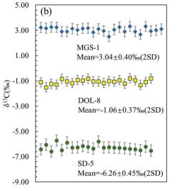
Fig. 6 External reproducibility of the C isotope analyses for MGS-1, DOL-8 and SD-5 (b) with the line scan ablation positions marked on MGS-1 (a).
