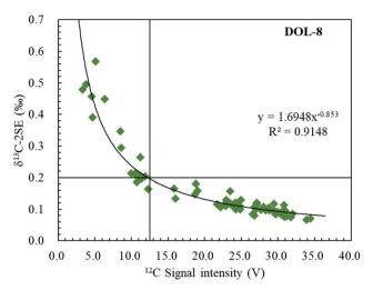
Fig. 5 Internal precisions of  $\delta^{13}$ C (2SE) measured by femtosecond laser ablation MC-ICP-MS on DOL-8, as a function of signal intensity of  $^{12}$ C (volts). It demonstrated that the measurement repeatability of the  $\delta^{13}$ C ratio (SE) is an exponential function of the  $^{12}$ C intensity.
