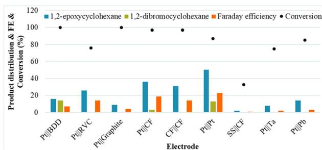
**Fig. 1** Product distribution with various electrodes. Reaction conditions: cathode||anode, constant current of  $10 \text{ mA cm}^{-2}$ , **1a** (50 mM), NaBr (1.0 eq.), MeCN/ $\text{H}_2\text{O}$  (4 : 1, 6 ml), room temperature, 3 h. Yield was determined by GC analysis using octane as the external standard compared with the desired cyclohexene oxide.
