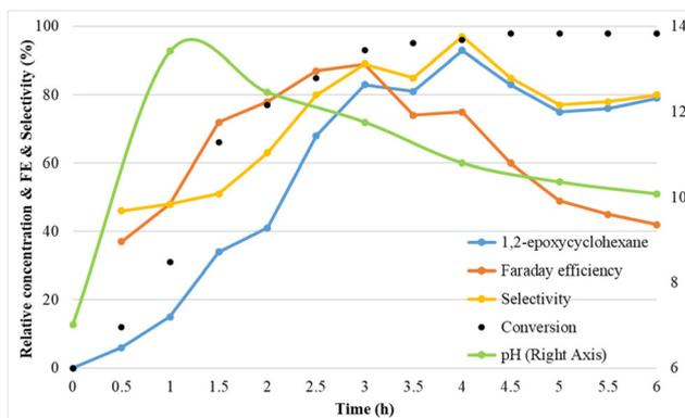
**Fig. 4** Reaction conditions: Pt as anode and Pt as cathode, constant current of  $7.5 \text{ mA cm}^{-2}$ , **1a** (75 mM),  $\text{Et}_4\text{NBF}_4$  (2 eq.), NaBr (1.5 eq.), MeCN :  $\text{H}_2\text{O}$  (3 : 2, 6 ml), room temperature.
