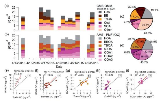
Fig. 7 AMS-PMF and OMM-CMB factors (Islam et al., 2020) OC averages from overlapping sample periods are from NAMaSTE1, Kathmandu Nepal, April 2015. OMM-CMB OC (a) and AMS-PMF OC average factors (b) shown are on the CMB time scale. Scatter plots of OMM-CMB (c) and AMS-PMF OC (d) average mass fractions compare well PMF and CMB factors HOA and traffic (e), BBOA and biomass (f), TBOA and trash (g), sLOA and coal (h), OOA and SOA with other (i) are shown as AMS-PMF OA results converted to OC.
