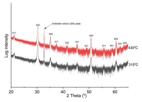
Fig. 3 The  $\theta$ -2 $\theta$  XRD analysis of deposited films at 315 °C (50 nm thick) and 430 °C (96 nm thick), showing polycrystalline cubic In<sub>2</sub>O<sub>3</sub> films.
