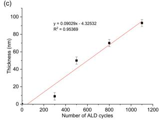
Fig. 2 (a) Growth per cycle behaviour of 4 and  $H_2O$  pulses at 290 °C on Si (100). (b) Growth dependence on process temperature using a 4 s pulse of 4 and 3 s pulse of  $H_2O$  on Si(100). (c) Growth behaviour of 4 at 290 °C dependent on the number of cycles using a 4 s pulse of 4 and 3 s pulse of  $H_2O$  on Si(100).
