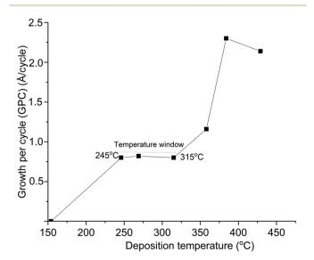
Fig. 7 Growth per cycle vs. deposition temperature for ALD of  $In_2O_3$  using 1 and  $H_2O$  in our ALD reactor, which does not have stop flow mode.
