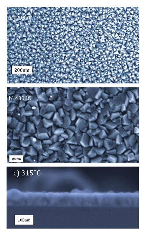
Fig. 4 SEM micrographs for films deposited at (a) 290 °C, (b) 430 °C and at (c) 315 °C.
