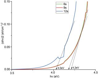
Fig. 6 Tauc plots for estimating the optical band gaps of  $In_2O_3$  films deposited with different  $H_2O$  pulse times.
