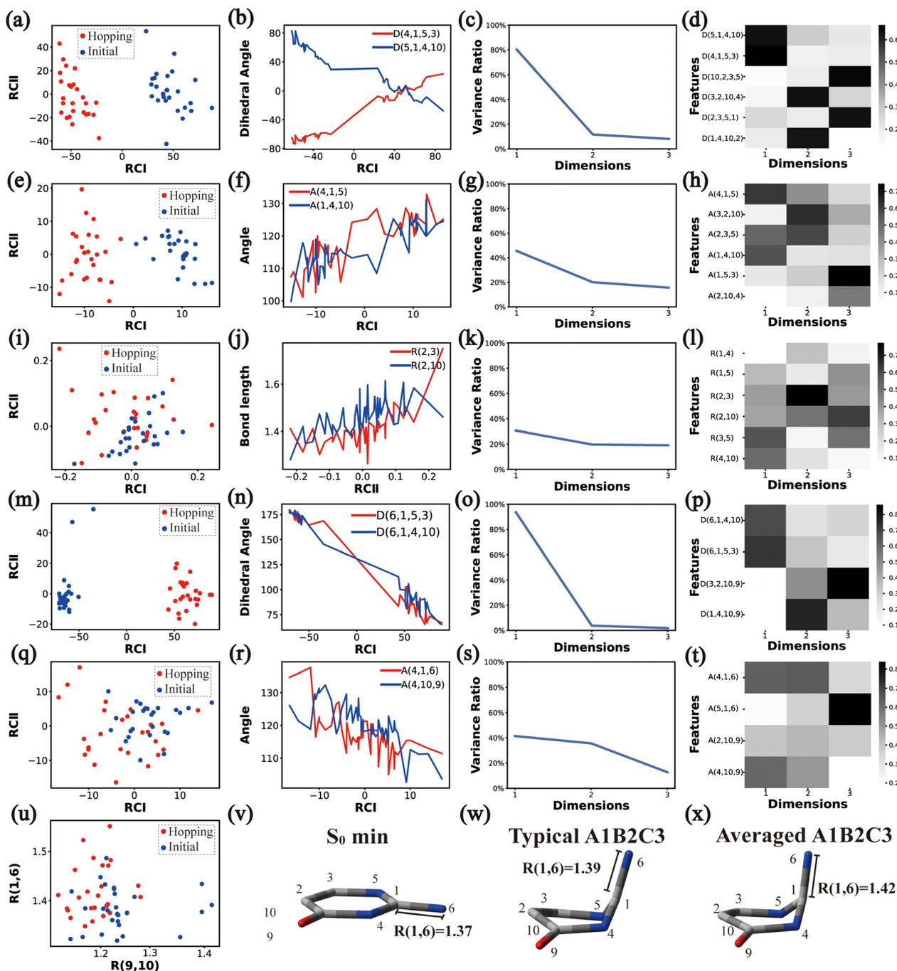
Fig. 5 The analysis results of Cluster **A1B2C3**. (a)–(d), (e)–(h), (i)–(l), (m)–(p) and (q)–(t) The PCA results of  $D_{\text{ring}}$ ,  $A_{\text{ring}}$ ,  $R_{\text{ring}}$ ,  $D_{\text{eg}}$  and  $A_{\text{eg}}$ . (u) The distributions of  $R(9,10)$  and  $R(1,6)$ . (v)–(x) Represent the  $S_0$  minimum, the typical and the averaged structures, respectively.
