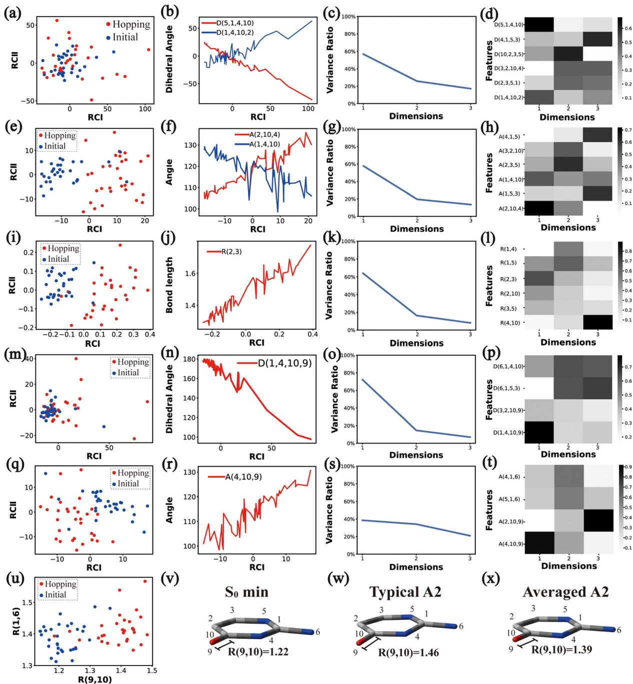
Fig. 7 The analysis results of Cluster **A2**. (a)–(d), (e)–(h), (i)–(l), (m)–(p) and (q)–(t) The PCA results of  $D_{\text{ring}}$ ,  $A_{\text{ring}}$ ,  $R_{\text{ring}}$ ,  $D_{\text{deg}}$  and  $A_{\text{deg}}$ , respectively. (u) The distributions of  $R(9,10)$  and  $R(1,6)$ . (v)–(x) Represent the  $S_0$  minimum, the typical structures and the averaged structures, respectively.
