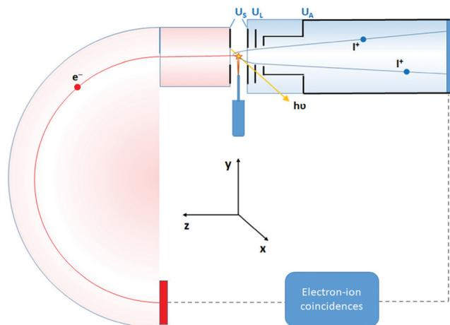
Fig. 1 Schematics of the electron–ion coincidence experiment at the Gas-phase Endstation (GPES).
