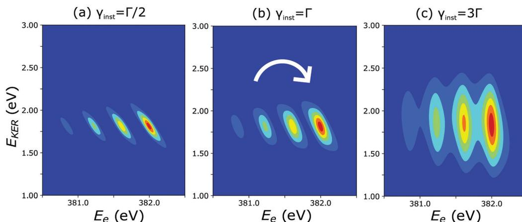
Fig. 10 Theoretical 2D plots of  $E_{\text{KER}}$  as a function of  $E_e$  calculated by eqn (8): the dispersion of vibrational lines ‘rotates’ clockwise with increase of the ratio  $\gamma_{\text{inst}}/\Gamma$  (see text for more details).
