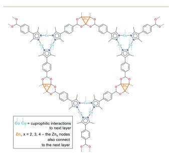
**Scheme 2** Common features of the structures of **1–3** with  $Zn_x$  nodes of different nuclearities (x = 2-4) and the trigonal  $\{Cu_3^I(mpba)_3\}^{3-}$  nodes giving a hexagonal-ring layer. Both the  $Zn_x$  nodes and the cuprophilic interactions from  $\{Cu_3^I(mpba)_3\}^{3-}$  connect to the next layer.
