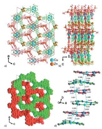
Fig. 8 View along the hexagonal channels of the two interpenetrating 3D-frameworks in 3 as (a and b) wire-frame, two projections and (c) space-filling modes. Network A in red with the Zn<sub>3</sub>-SBU and network B in green with the Zn<sub>4</sub>-SBU (*cf.* Fig. 7). (d) Stacking of the  $\{Cu_3^l(pz)_3\}$  moieties in 3 with  $Cu^l\cdots Cu^l$  contacts (in cyan, distances in Å) between the layers of the interpenetrating frameworks.
