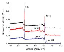
Fig. 1 Survey spectra of GO (black line), GO-NaOH (red line) and GO-Lys
