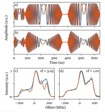
Fig. 4 Cartesian representations of the CHORUS sequence: (a) without and (b) with compensation. Normalised experimental excitation spectra of bisnitroxide (Scheme 1) obtained with the CHORUS sequence (red) are shown in (c) before and (d) after amplitude optimisation and hardware compensation and are compared with the reference field-sweep spectrum (blue). The corresponding values of the cost function (cf) are shown in both cases.
