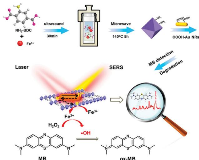
Fig. 9 Schematic diagram of the preparation of Au NRs/Fe-MOFs for methylene blue *in situ* catalytic degradation and SERS detection. Reproduced from ref. 138 with permission from American Chemical Society, copyright 2022.
