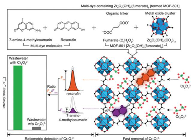
Fig. 5 Schematic of the ratiometric detection and simultaneous removal of  $\text{Cr}_2\text{O}_7^{2-}$  using multi-dye (resorufin and 7-amino-4-methylcoumarin) containing MOF-801. Reproduced from ref. 115 with permission from Elsevier Inc, copyright 2019.
