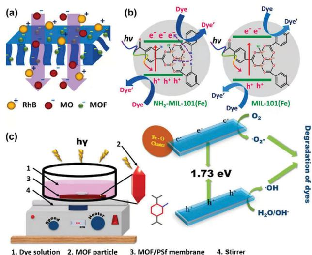
Fig. 10 Schematic illustration of (a) rejection and (b) photocatalytic degradation of dye molecules over the NH<sub>2</sub>-MIL-101(Fe) and MIL-101(Fe) MOF-integrated membranes and (c) pictorial illustration of degradation setup and its mechanism. Reproduced from ref. 139 with permission from Elsevier Inc, copyright 2022.
