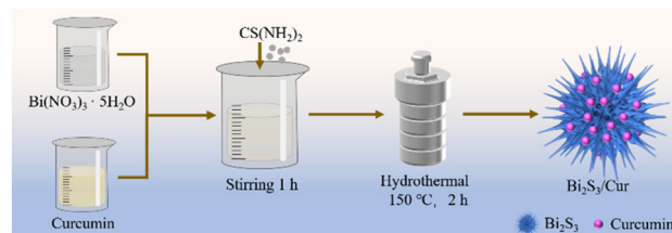
Scheme 2 Schematic diagram of Bi 2 S 3 /Cur hybrid material synthesis.
