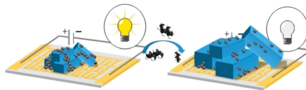
Fig. 5 Switchable MIL-53-carbon additive composite for CO 2 sensing. 25
