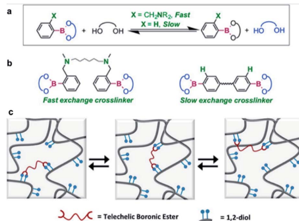
Fig. 4 (a) Kinetics of the exchange reaction of boronic esters according to their neighboring functional groups. (b) Transesterification reaction using boronic ester as a cross-linking agent. (c) Schematic of the boronic ester exchange reaction. Reproduced from ref. 55 with permission from the ACS.
