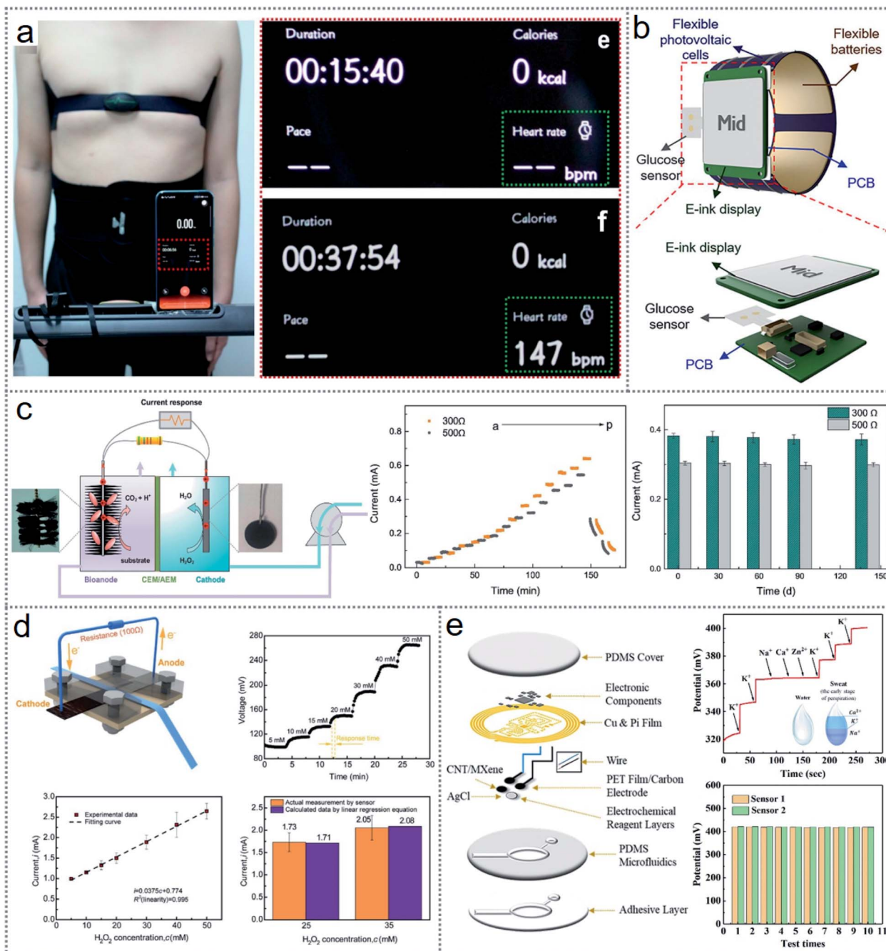
Fig. 12 Applications of electrochemical effect-based redox devices. (a) Optical image of the wireless heartbeat sensing device. (b) Schematic of the architecture of glucose monitoring sensor integrated with a self-powered smartwatch. (c) Schematic of the microbial fuel cell (MFC)-based electrochemical sensor and performances of the device. (d) Schematic of the membraneless microfluidic cell (MMFC) sensor and detection performances of the device. (e) Schematic of the battery-free integrated skin mountable electrochemical sensors and the sensing performance of the device. Figures reproduced with permission from: (a) ref. 25, © 2020, the American Chemical Society; (b) ref. 122, © 2019, the American Chemical Society; (c) ref. 123, © 2019, Elsevier; (d) ref. 124, © 2020, the American Chemical Society; and (e) ref. 127, © 2021, Elsevier.
