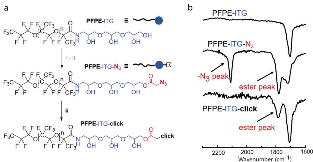
Fig. 4 (a) Post-modification of PFPE-ITG by esterification: (i) bromoacetic acid, EDC-HCl, DMAP, DMF-HFE7500; (ii) NaN<sub>3</sub>, DMF-HFE7500; and (iii) DBCO-PEG4-Biotin, CH<sub>3</sub>OH-HFE7100. (b) FT-IR spectra showing the presence of azide and ester in the modified PFPE-ITG-N<sub>3</sub> surfactant, absence of both in the pristine surfactant, and disappearance of the azide signal after the click reaction.
