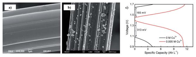
Fig. 12 SEM images of (a) original graphite felt and (b) the graphite felt decorated with copper nanoparticles. (c) Charge and discharge curves of VRFBs employing electrolytes containing different Cu<sup>2+</sup> concentrations at 300 mA cm<sup>-2</sup>. Extracted from ref. 361.
