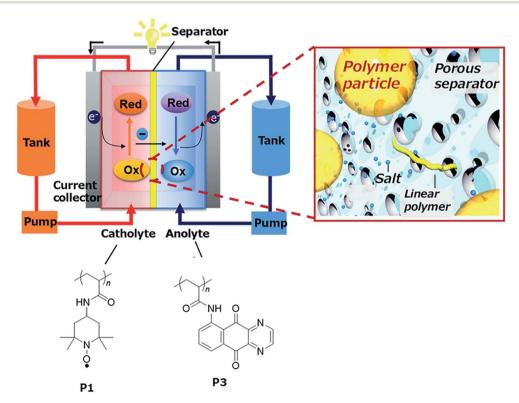
Scheme of the RFB based on organic redox-active polymer nanoparticles developed by Hatakeyama-Sato et al. extracted from ref. 221.
