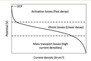
Fig. 17 Generalized polarization curve for a VRB indicating the dominant source of overpotential in each region.
