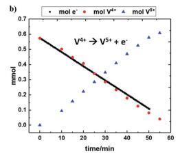
Fig. 19 (a) Monitoring of a VRFB during charge by UV-Vis. (b) Evolution of the number of moles of reduced (red) and oxidized (blue) species and the number of moles of electrons removed electrochemically (black line). Extracted from ref. 471.
