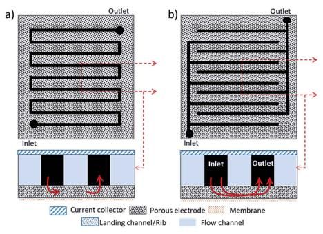
Fig. 14 Cross section views of the flow channels over the porous electrode using: (a) serpentine flow field (IFF); and (b) interdigitated flow field (IFF) (adapted from ref. 11).
