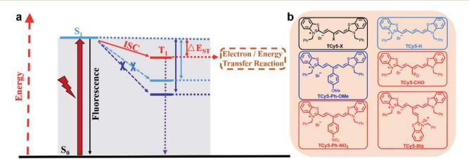
Fig. 1 (a) Schematic illustration of the strategy for our NIR excited TCy5 system via the optimization of the singlet-triplet energy gap ( $\Delta E_{st}$ ) by a meso-substitution group (X). (b) Molecular structures of the photosensitizers (TCy5-H, TCy5-Ph-MeO, TCy5-Ph-NO<sub>2</sub>, TCy5-CHO and TCy5-Btz) in this study.
