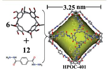
Fig. 3 Schematic illustration of the assembly of the [6+12] octahedron based on C4RACHO and the linear terephthalohydrazide linker and its X-ray crystal structure. The hydrogen atoms and *iso*-butyl groups are omitted for clarity.
