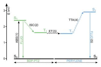
Fig. 5 Simplified Jablonski diagram illustrating the main excited states' energy levels and processes involved in TTA upconversion. In this example, A = BDP-PTZ and B = perylene.
