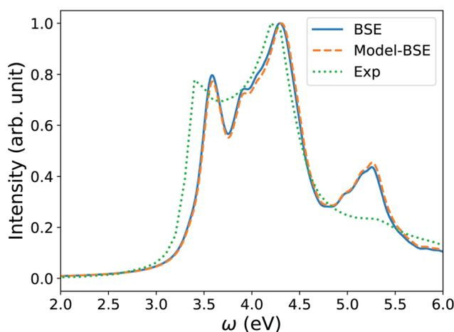
Fig. 4 Absorption spectrum of crystalline Si computed by solving the Bethe–Salpeter equation (BSE) starting from PBE<sup>75</sup> wavefunctions, using a 2-atom cell and  $12 \times 12 \times 12$   $k$ -point sampling (blue line). The orange dashed line (Model-BSE) shows the same spectrum computed using a diagonal dielectric matrix with diagonal elements equal to  $\epsilon_{\infty} = 12.21$  (see text). Experimental results<sup>86</sup> are shown by the green dotted line.
