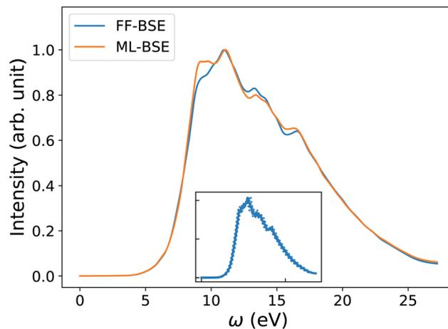
Fig. 7 Average spectra of  $\text{Si}_{35}\text{H}_{36}$  obtained by solving the Bethe–Salpeter equation (BSE) in finite field (FF) and using machine learning techniques (ML). Results have been averaged over 10 snapshots obtained from first principles simulations at 500 K. The variability of the FF-BSE spectra within the 10 snapshots is shown in the inset. See also Fig. S21 of the ESI† for the same variability when using ML-BSE.
