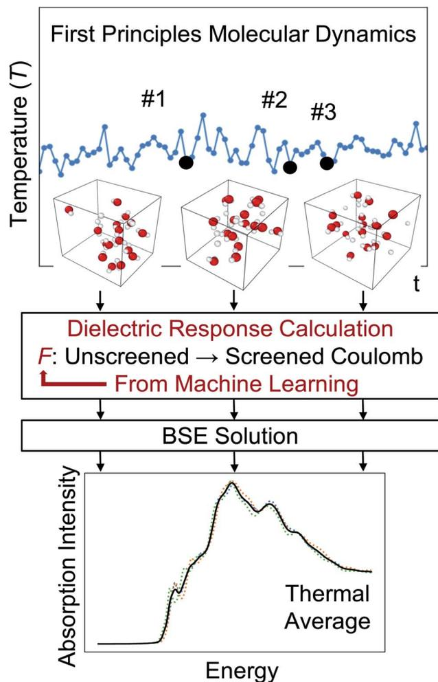
Fig. 1 Illustration of the strategy to predict absorption spectra at finite temperature based on the solution of the Bethe–Salpeter equation (BSE) and machine learning techniques.  $F$  is the mapping obtained by machine learning.
