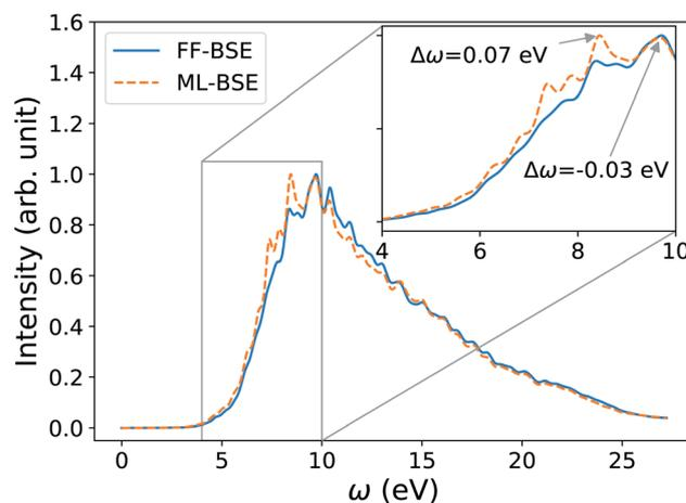
Fig. 8 Accuracy of the  $\text{Si}_{87}\text{H}_{76}$  spectrum obtained from ML-BSE by applying a convolutional model with filter size (7, 7, 7), trained from  $\text{Si}_{35}\text{H}_{36}$ . The RMSE value between the FF-BSE and ML-BSE spectra is 0.033.
