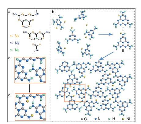
Scheme 1 (a) Molecular structure of heptazine-based PCN. (b) Proposed schemes of thermal polymerization of heptazine units with Ni-N coordination. Regional schemes of (c) PCN with hydrogen bonding between terminal -NH2 and -NH- groups, and (d) PCN with broken hydrogen bonding with single-atom Ni as the terminating agent.
