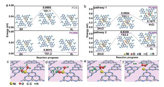
Fig. 6 Reaction pathways of (a) water reduction to  $H_2$  and (b) water oxidation to  $H_2O_2$  (top) and  $O_2$  (down) for PCNNi (single-atom Ni coordinated with sp<sup>2</sup> NA atoms). (c–f) Proposed mechanisms of photocatalytic pure water splitting into  $H_2$  and  $H_2O_2$  for PCNNi (single-atom Ni coordinated with sp<sup>2</sup> NA atoms).
