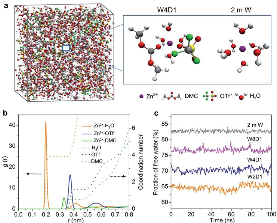
Fig. 2 MD studies of the Zn<sup>2+</sup> solvation structure. (a) Snapshot of the MD simulation cell for the W4D1 electrolyte, and the representative Zn<sup>2+</sup> solvation structures in W4D1 and 2 m W electrolytes. (b) RDFs of Zn-O (H<sub>2</sub>O), Zn-O (DMC) and Zn-O (OTf<sup>-</sup>) pairs, and the coordination number in the W4D1 electrolyte. (c) Fraction of free water (not solvating to Zn<sup>2+</sup>) in the H<sub>2</sub>O + DMC electrolytes with a 100 ns simulation time.
