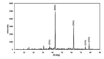
Fig. 2 The XRD pattern of the synthesized MgO.
