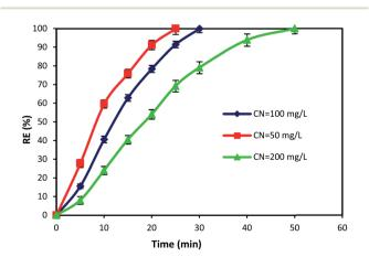
Fig. 8 Effects of contact time and initial cyanide concentration on the removal of cyanide by MgO/O $_3$ /PS process.
