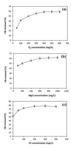
Fig. 7 The effects of ozone concentration (a) and MgO dosage (b) in MgO/O<sub>3</sub> process and PS concentration (c) in MgO/O<sub>3</sub>/PS process (MgO =  $500 \text{ mg L}^{-1}$  in (a), ozone =  $400 \text{ mg h}^{-1}$  in (b), time = 30 min) (MgO =  $600 \text{ mg L}^{-1}$ , ozone =  $400 \text{ mg L}^{-1}$ , time = 20 min in (c)).
