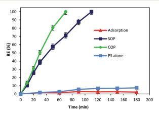
Fig. 6 Contribution of adsorption, SOP, COP and PS alone on cyanide removal (cyanide concentration: 100 mg  $L^{-1}$ , MgO concentration: 500 mg  $L^{-1}$ , ozone concentration: 200 mg  $L^{-1}$ , PS concentration: 200 mg  $L^{-1}$ , pH = 11, reaction time: 180 min).
