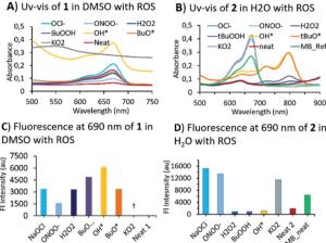
Fig. 2 Optical properties of MB-BHT (25 nmol mL<sup>-1</sup>) after treating sufficient amount of ROS (>5 equiv.). Fluorescence emission (concentration 12 nmol mL<sup>-1</sup>) at the maximum of 689 nm for excitation at 645 nm (†: due to fast decomposition of the formed MB).
